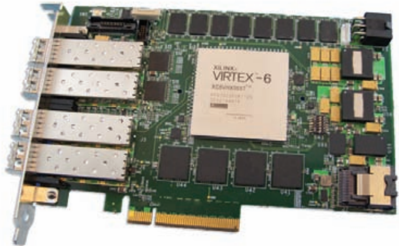
Figure 6 – The V5022 is a single-slot, half-length card deployed worldwide in financial trading systems.
