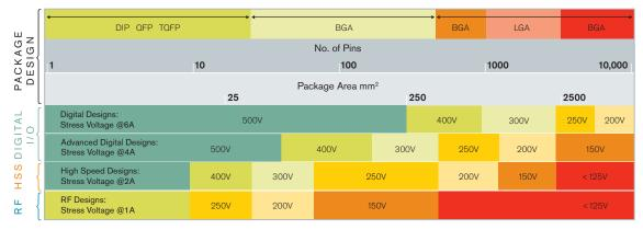
CDM package map projected for 22nm designs. Products with >1000 pins or 1200mm<sup>2</sup> area would be limited to <150V CDM passing voltage for all HSS and RF designs.
