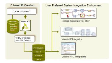
Xilinx All Programmable devices without the need to manually create RTL. Vivado HLS is part of the Vivado Design Suite, System Edition.
