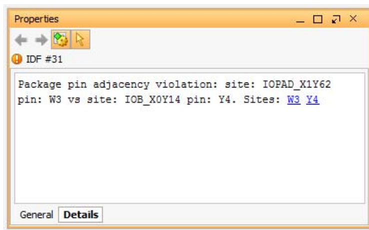
Figure 6: Pin Adjacency Violations Highlighted in Package Window
