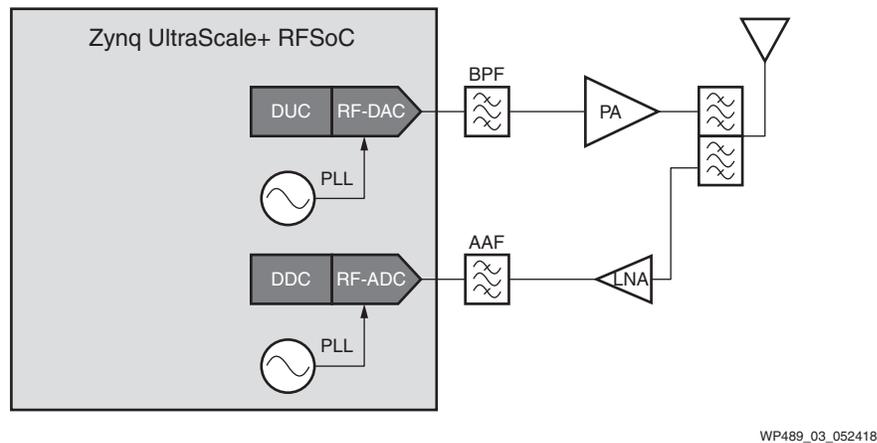
Figure 3: Software Defined Radio Using Zynq UltraScale+ RFSoc
