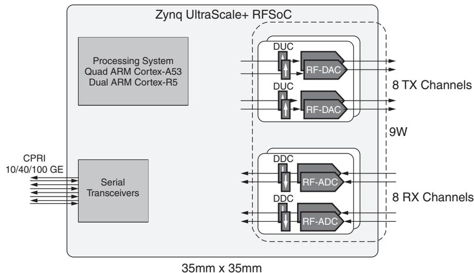
Figure 5: RF Front End Based Zynq UltraScale+ RFSoc
