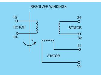
Figure 1 - Excitation to the rotor of a resolver
