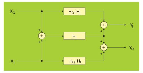
Figure 5 – Implementation architecture of a complex filter
