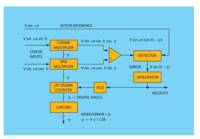
Figure 2 - Resolver-to-digital converter (RDC) block diagram
