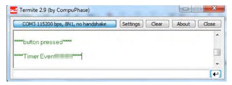
Figure 3 – This screen shows an example of the GPIO and timer interrupt event outputs.
