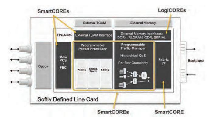
Figure 3 – With SDNet, companies can create a highly integrated All Programmable line cards.
