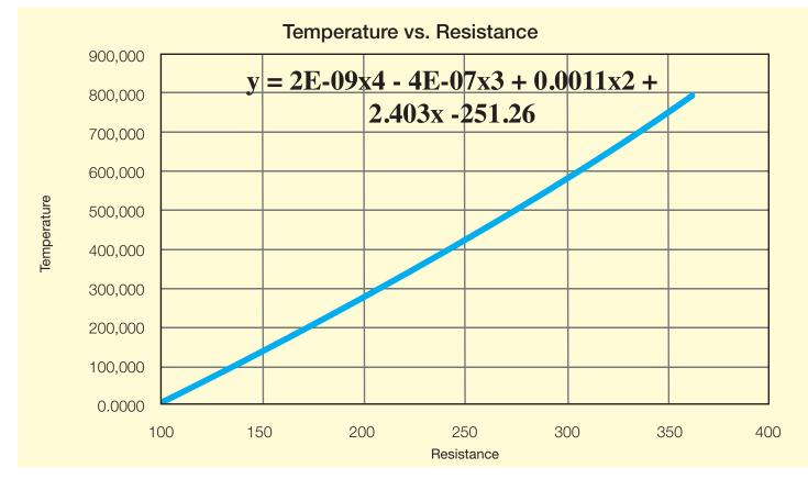
Figure 2 – Trend line and polynomial equation for the temperature transfer function
