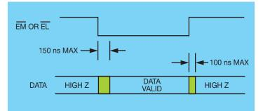
Figure 7 – ENABLE timing
