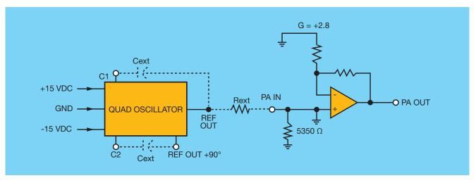
Figure 4 – Block diagram of the OSC-15802 reference oscillator
