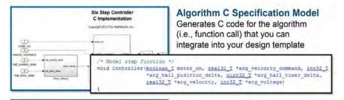
Six Step Commutator And Peripherals
