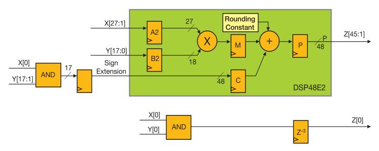
Figure 2 – A 28x18-bit signed multiplication with convergent rounding capability of the output
