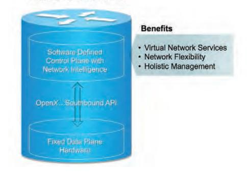
Figure 1 – Today's software-defined networks separate the control and data planes but still have fixed data planes, minimal differentiation and short life cycles.
