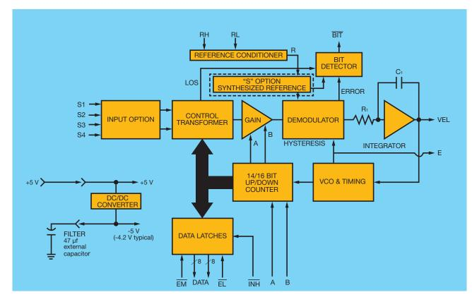
Figure 3 – SD-14620 block diagram (one channel)
