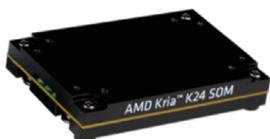
K24 SOM pictured with fully enclosed thermal solution
