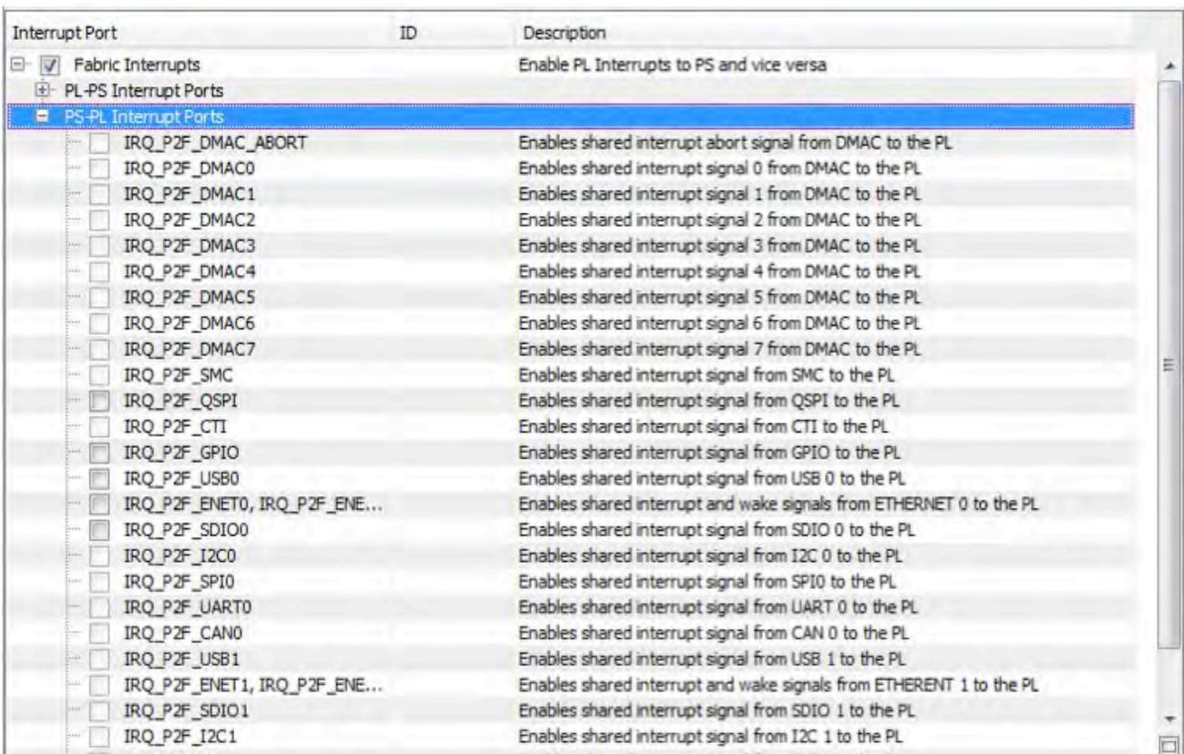
Figure 2 – These are the interrupts available between the processing system and the programmable logic.
