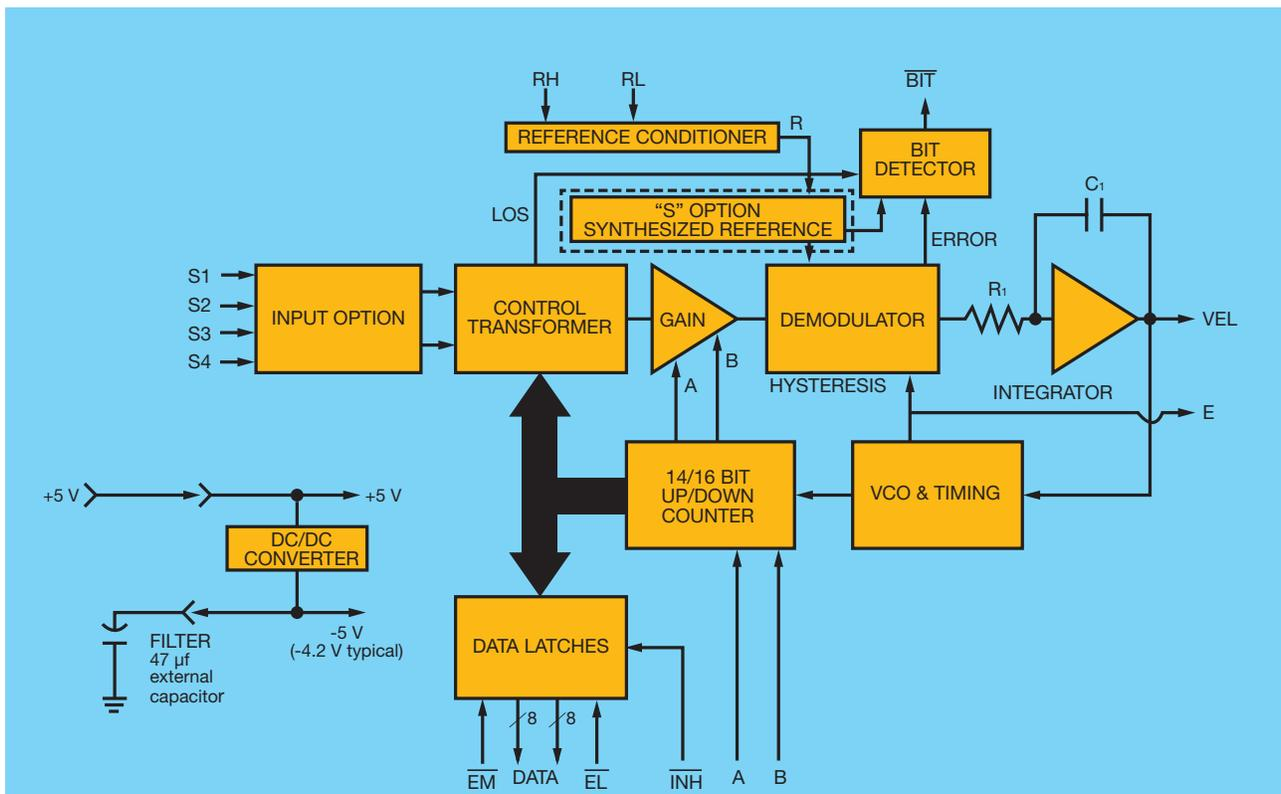
Figure 3 – SD-14620 block diagram (one channel)
