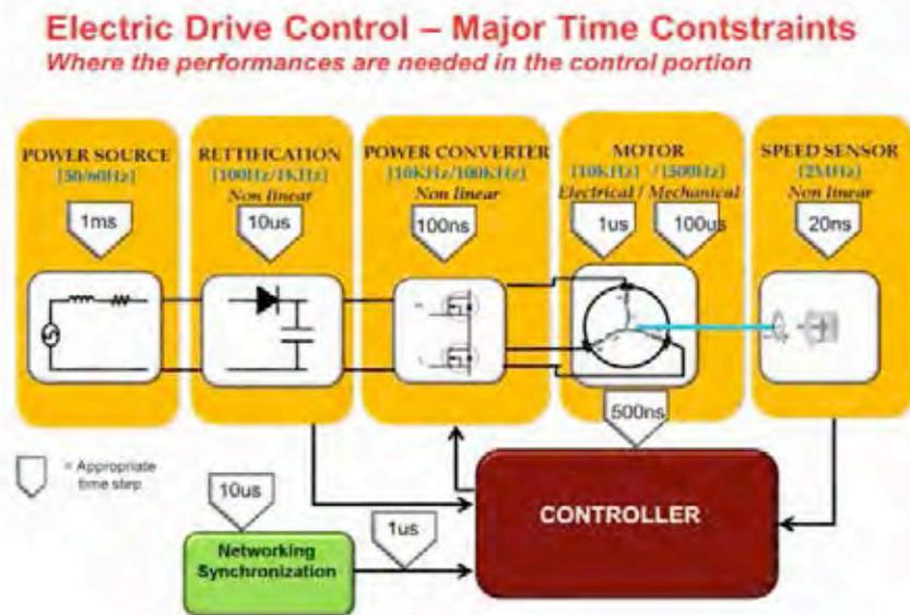
Figure 2 – Major time constraints of electrical drive controllers
