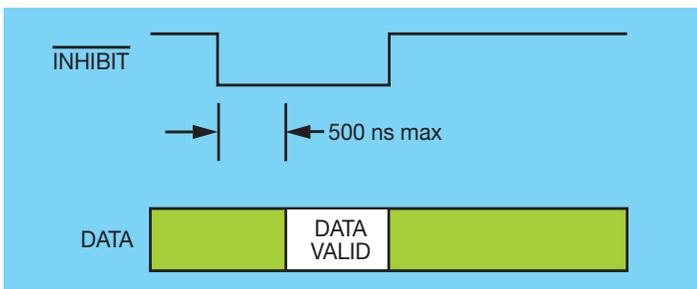
Figure 6 – INHIBIT timing
