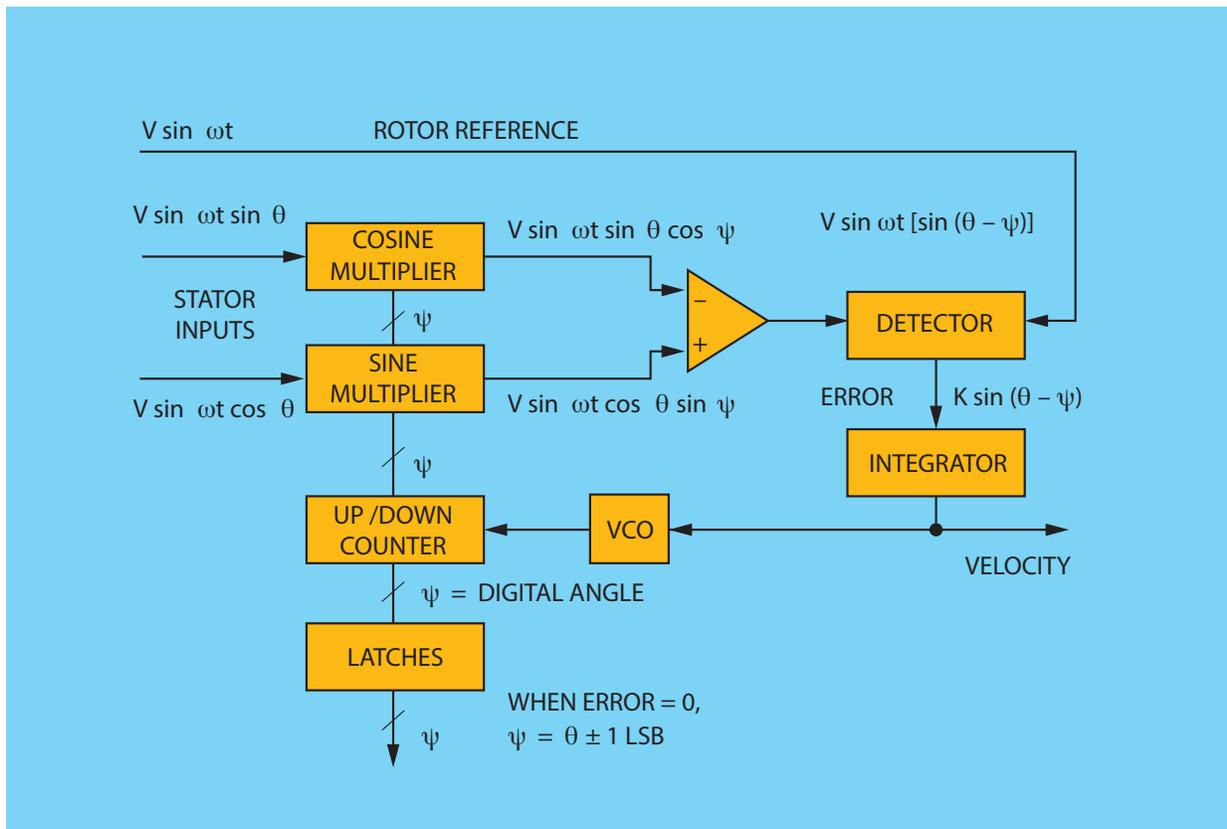
Figure 2 – Resolver-to-digital converter (RDC) block diagram
