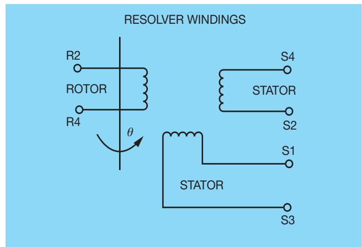
Figure 1 – Excitation to the rotor of a resolver
