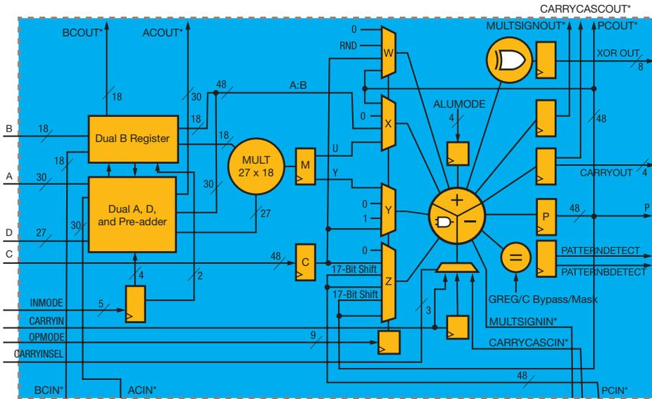
\* These signals are dedicated routing paths internal to the DSP48E2 column. They are not accessible via general-purpose routing resources.
