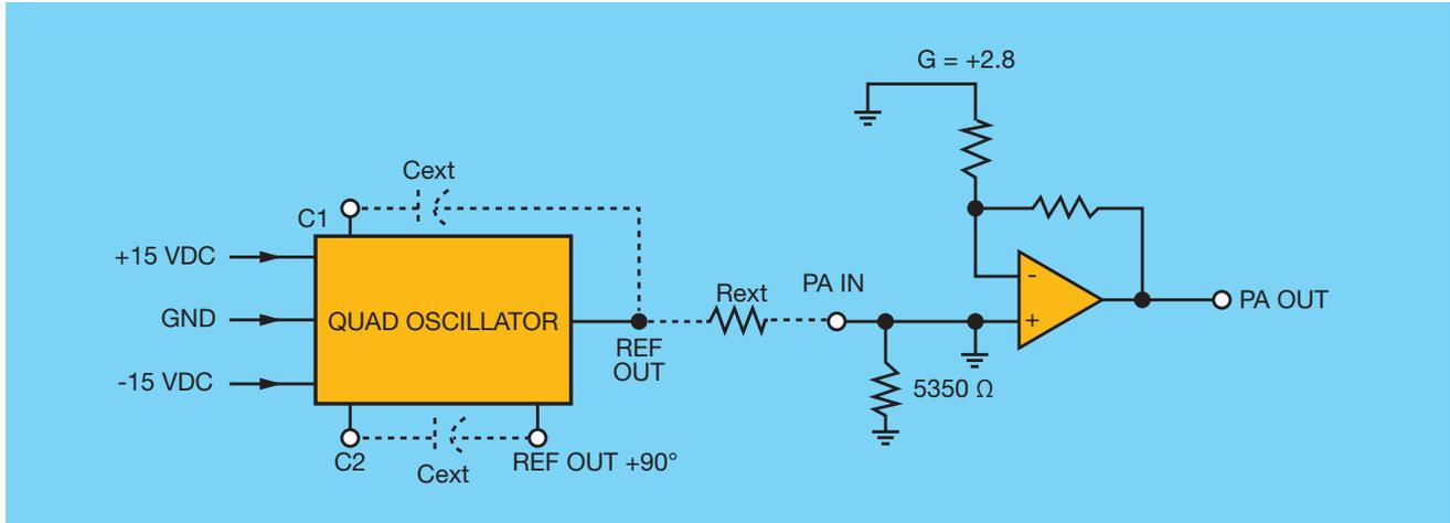
Figure 4 – Block diagram of the OSC-15802 reference oscillator
