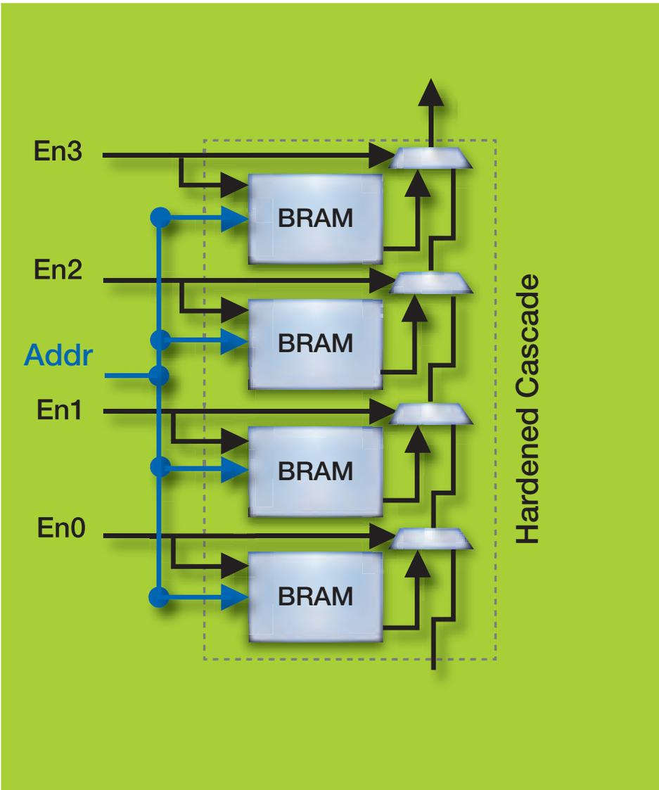
Figure 6 – BRAM cascade on UltraScale devices
