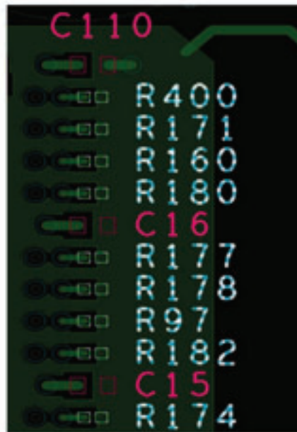
Figure 7: V_{TT} Capacitor Placement
