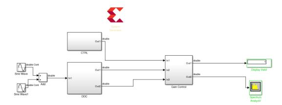
When this design is complete, the logic within each subsystem will execute at different clock frequencies. The clock domains might not be synchronous with each other. There is presently nothing to prevent incorrect data being sampled between one subsystem and another subsystem.
