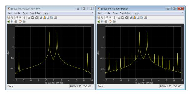
The results are shown above, on the right hand side (in the Spectrum Analyzer SysGen window), and differ slightly from the original design (shown on the left in the Spectrum Analyzer FDA Tool window). This is due to the quantization and sampling effect inherent when a continuous time system is described in discrete time hardware.
