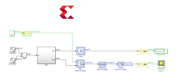
11. Select the components in the output path and create a subsystem named Gain Control.
