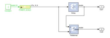
This will create an output strobe on Out2 which will be active for one cycle when the input changes, and be used as the write-enable from CTRL to the Gain Control (the FIFO block at the top level).
