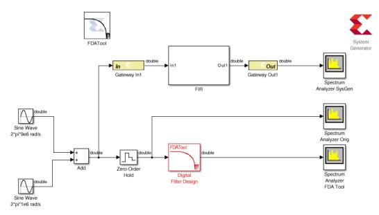
In the previous figure, both the input and output of instance FIR are of type double.
