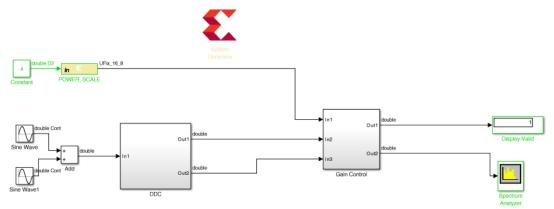
12. Finally, select the Gateway In instance **POWER\_SCALE** and **Constant** to create a new subsystem called CTRL. The final grouped design is shown in the following figure.
