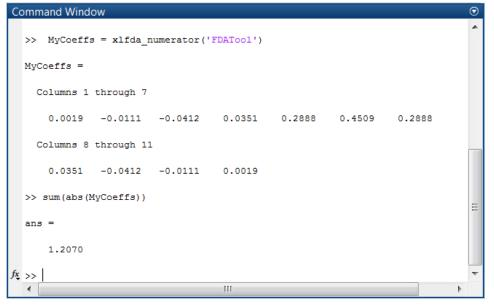
Taking into account the positive and negative values of the coefficients the maximum gain possible is 1.2070 and the output signal should only ever be slightly smaller in magnitude than the input signal, which is a 16-bit signal. There is no need to have 15 bits (43-28) of data above the binary point.
