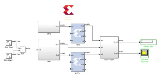
You will now connect up the control logic signals to ensure the data is safely passed between domains.
