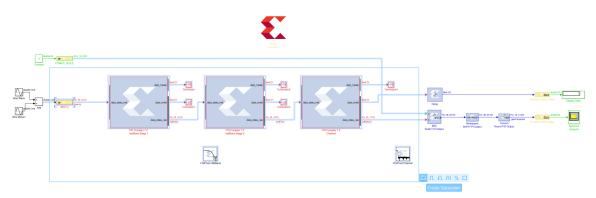
10. Select the instance name subsystem and change this to DDC to obtain the design shown.
